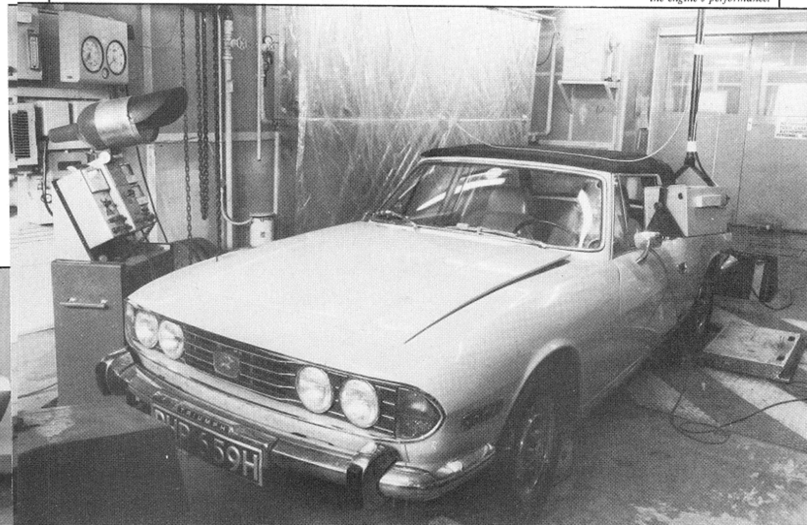
A pre-production Stag on a rolling road test. The box by the driver's door gives a readout of the engine's performance.
